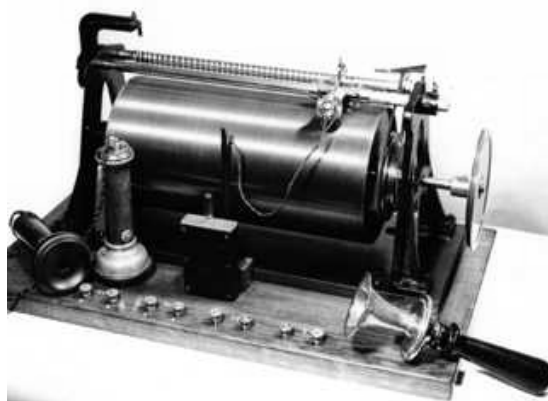
Figure 1.1: Early version of Poulsen's Telegraphone.
