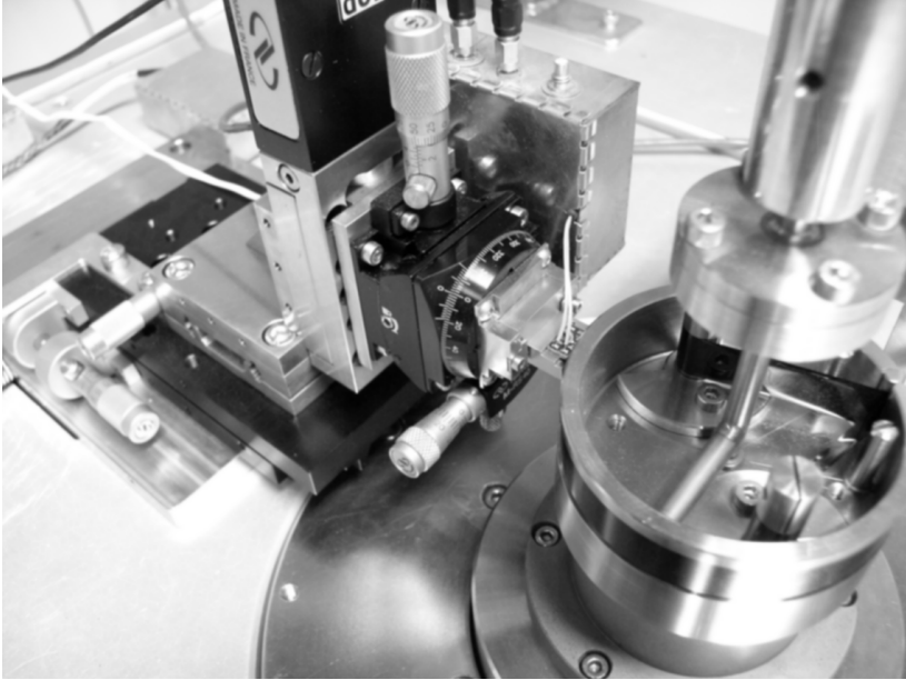
Figure 4.6: View of the upgraded tape-drum tester (drum and head positioning mechanism).
